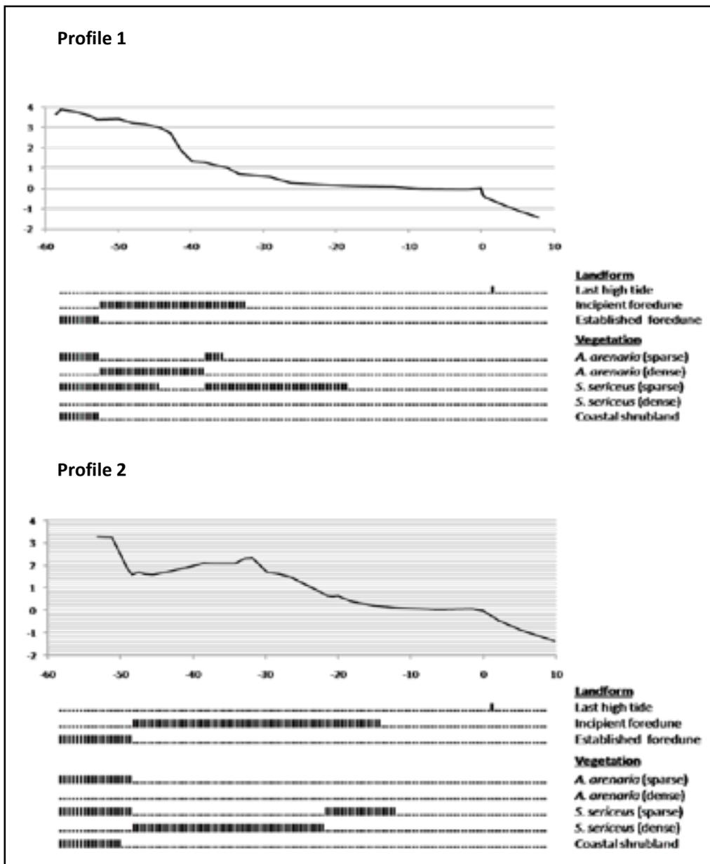
Figure 8.1: Example of laser surveyed shore-normal transects with relevant geomorphic and botanical features
