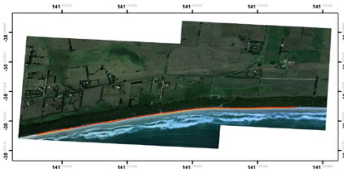
**Figure 8.4: Example of aerial photograph analysis to determine shoreline stability**
